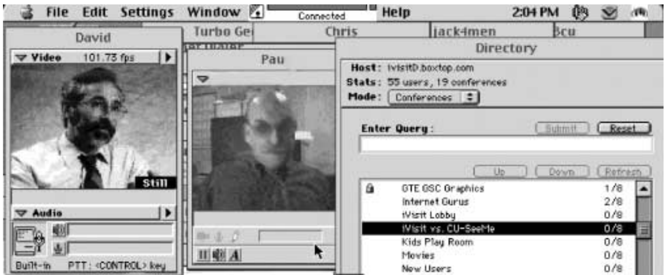
This is a computer screen snapshot of videoconferencing over the Internet. The pictures on the left are two individuals talking and seeing each other from different parts of the country. The box on the right lists the virtual room they are conversing in at the time.
